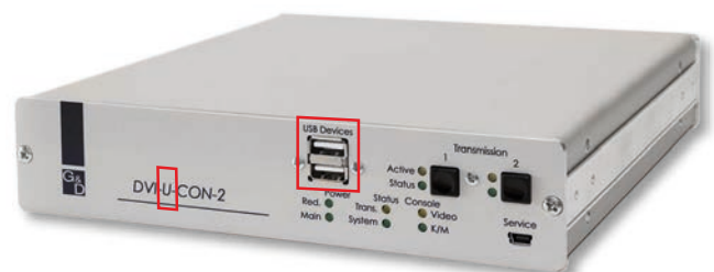
Front panel of DVI-U-CON-2 with interfaces for transparent USB transmission
