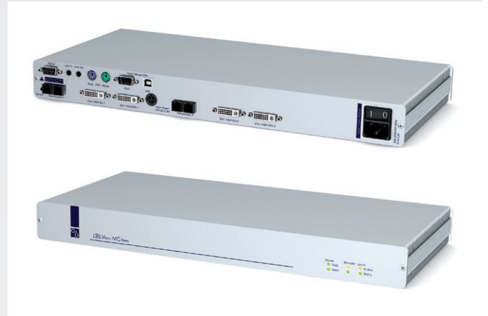
above: LwLVision(S)-MC2-AR-PC computer module below: LwLVision(S)-MC2-AR-CON user module
