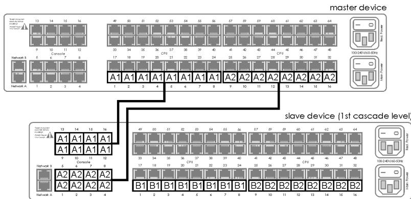
The **CPU** ports 1 - 16 of the master device are connected with one twisted pair cable each. Each of these cables is attached to a **Console** port of the slave device.
