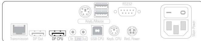
**DP CPU:** Use the *DP-Cable-M/M-2* cable to connect the computer's video output to this interface.
