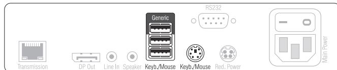
**NOTE:** Both the keyboard and the mouse of the console can either be PS/2 or USB devices.
