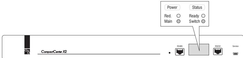
**Figure 3: Status displays at the front panel of the matrix switch**
