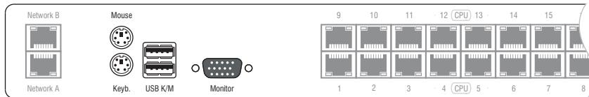
**Figure 2: Interfaces to connect the local console**
