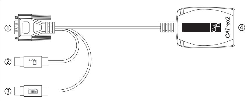
Figure 1: Legend of *CATpro2-PS/2* target module
