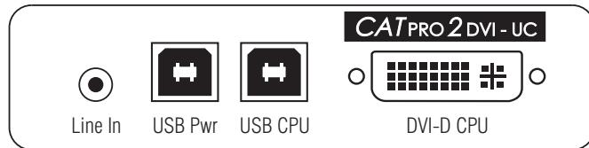
Figure 5: Front view of the CATpro2-DVI-Audio target module
