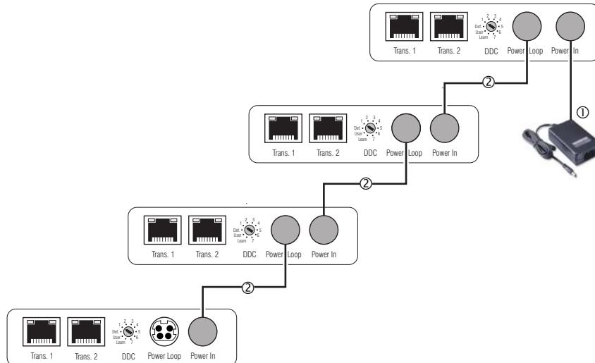
**Figure 8: Power Loop power supply of four devices via one power pack**
