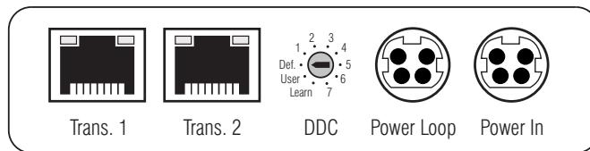
**Figure 6: Back view of the CATpro2-DVI-Audio target module**
