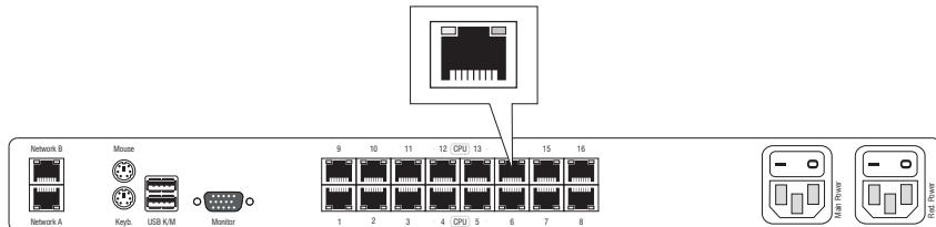
**Figure 4:** Status displays at the RJ45 interfaces of the matrix switch
