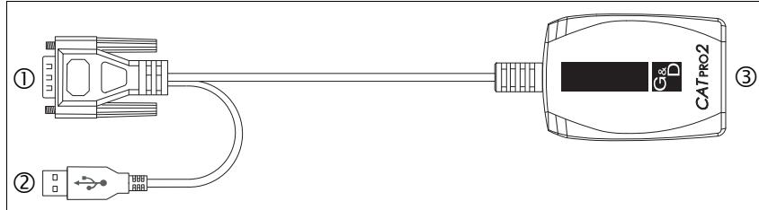
Figure 2: Legend of *CATpro2-USB* target module
