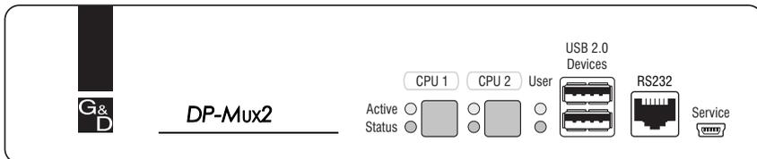
Figure 1: Front view of the KVM switch
