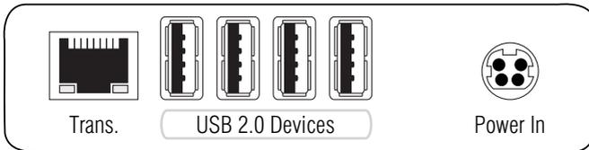
**Trans.:** Use a category 5e (or better) twisted pair cable to connect this interface to the *Dynamic Port* of the *USB/RS232 Main Channel* that is assigned to the console.
