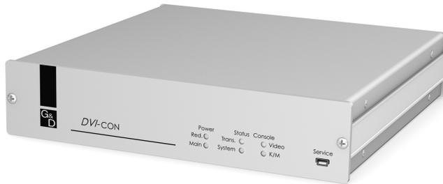
First connect the console devices (monitor, keyboard, mouse, and audio devices) to the user module. Then connect the user module to a matrix switch of the *DVICenter* series.
