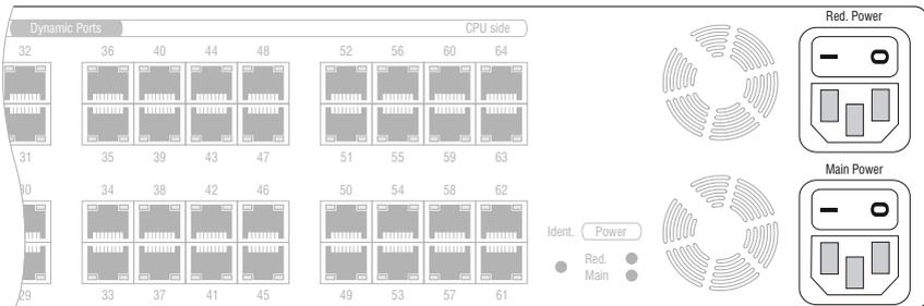
**Main Power:** Plug one of the supplied power cable in this interface. Connect the power cable with a power outlet and turn the power button on.
