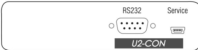
**RS232:** Connect the serial end device to this interface.
