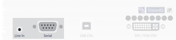
**NOTE:** By default, the KVM extender transfers audio data. The transmission of RS232 data is deactivated.
