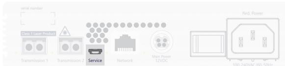
Debug, error and status messages can be displayed in a terminal emulator (e.g. *HyperTerminal* or *PuTTY*). Via a service menu, technicians have the ability to retrieve information about the device, temporarily disable the network filter rules, reset the device to factory settings, or perform a restart.
