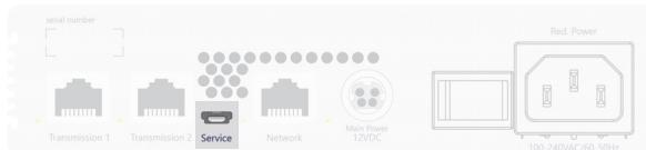
Debug, error and status messages can be displayed in a terminal emulator (e.g. *HyperTerminal* or *PuTTY*). A service menu gives technicians the option of reading out information about the device, resetting the device to the factory settings or performing a restart.
