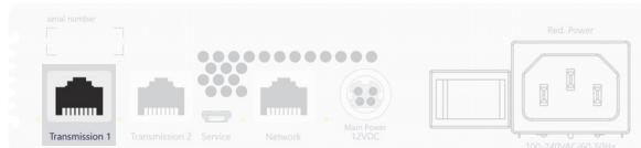
**Transmission 1:** Plug a category 6 (or better) twisted pair cable, which is available as accessory, into this interface. Connect the other end of the cable to the respective interface of the computer module or to one of the *Dynamic Ports* of a compatible matrix (see page 4).
