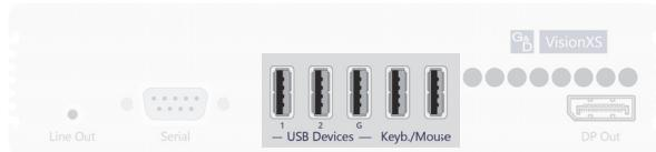
**Keyb./Mouse:** Connect the mouse and/or the keyboard of the console to this interface.
