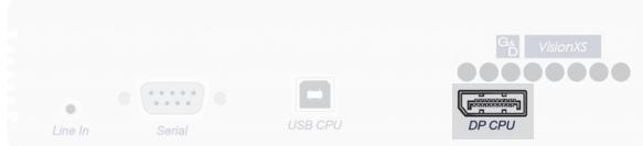
**DP CPU:** Use the *DP-Cable-M/M-2* cable to connect the computer's video output to this interface.
