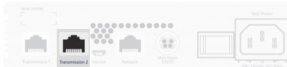
**Transmission 2:** Plug a category 6 (or better) twisted pair cable, which is available as accessory, into this interface. Connect the other end of the cable to the respective interface of the computer module.
