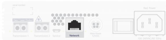
**NOTE:** If desired, connect this network interface to a local network. This enables you to access the **Config Panel** web application from this network and to send syslog messages to this network.
