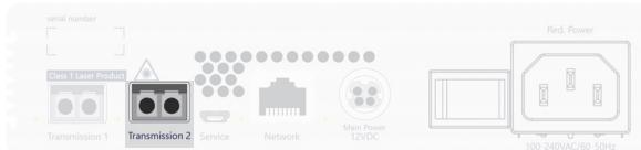
**IMPORTANT:** The device uses components with laser technology which comply with laser class 1.
