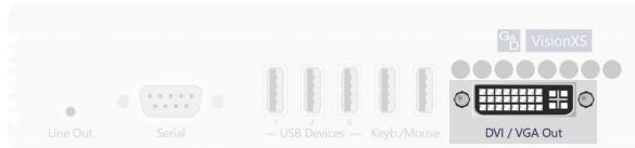
**DVI/VGA Out:** Connect the console monitor.
