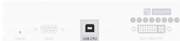
**USB CPU:** Use the **USB-AM/BM-2** cable to connect one of the computer's USB interfaces to this interface.
