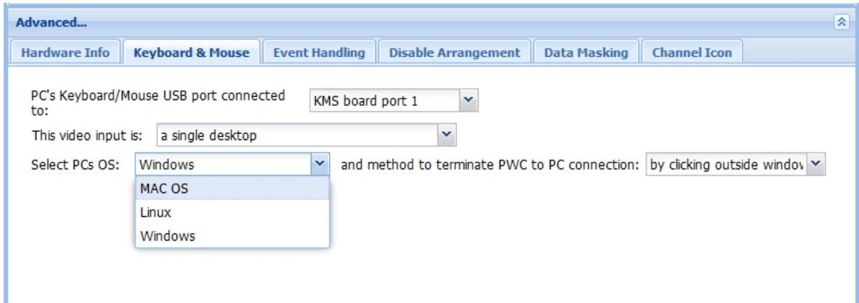
Figure: Keyboard & mouse tab for single desktop
