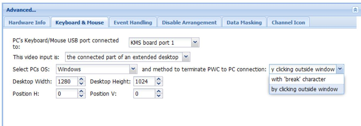
Figure: Keyboard & mouse tab for extended desktop
