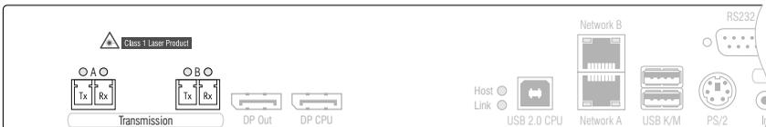
**IMPORTANT:** The device uses components with laser technology complying with laser class 1.
