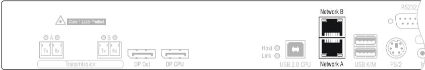
**NOTE:** If desired, connect the network interface to up to two local networks. Now you can not only access the **Config Panel** web application from those networks but also send syslog messages to those networks.
