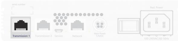
**Transmission 1:** Plug a category 6 (or better) twisted pair cable, which is available as accessory, into this interface. Connect the other end of the cable to the respective interface of the console module or to one of the *Dynamic Ports* of a compatible matrix (see page 4).
