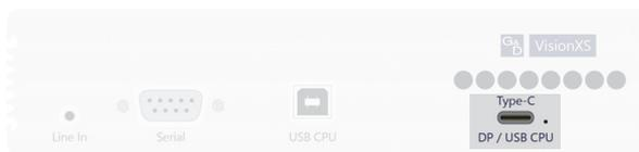
**Type-C DP/USB CPU:** Use the *TypeC-Cable-M/M-2* cable to connect one of the computer's USB interfaces to this interface.
