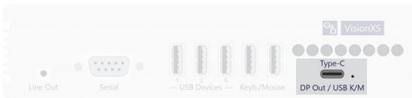
**Type-C/DP Out/USB K/M:** Connect the console monitor.
