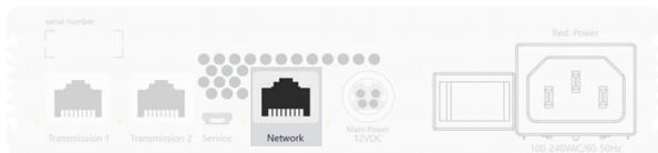
**NOTE:** If desired, connect this network interface to a local network. This enables you to access the **Config Panel** web application from this network and to send syslog messages to this network.
